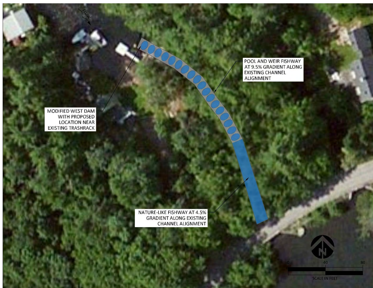
Figure 100. Schematic layout of a hybrid nature-like fishway and pool-and-weir fishway at West Dam.
