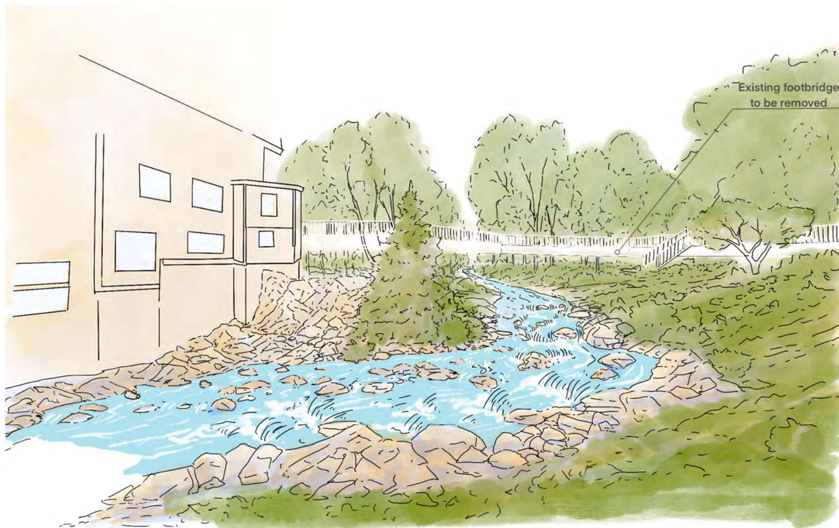
Figure 111. Ground-level rendering of the long-term conditions at the Knowlton Street dam site following dam removal, looking upstream from the dam location.
