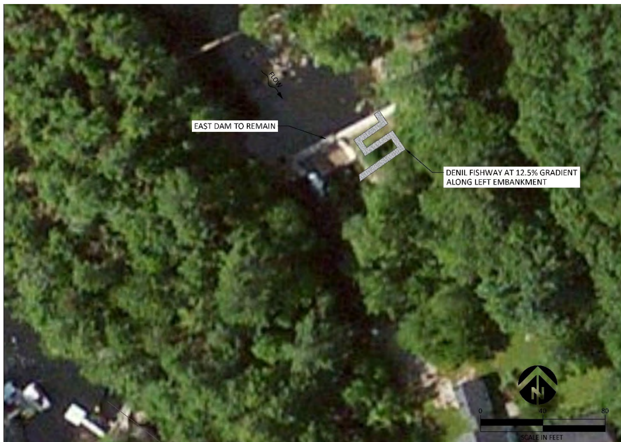
Figure 102. Schematic layout of a Denil fishway option at East Dam.
