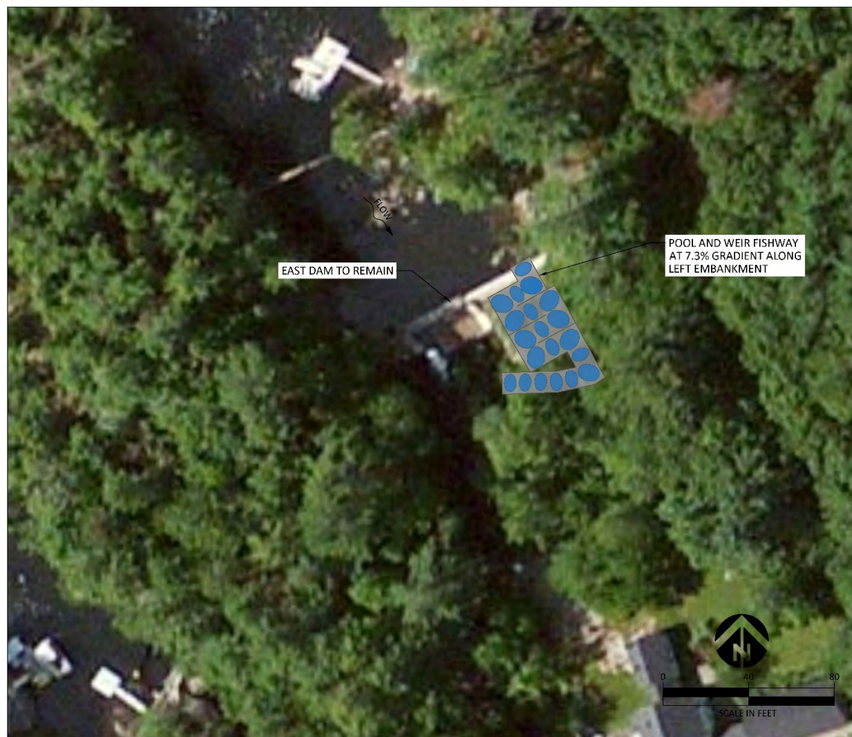
Figure 101. Schematic layout of a pool-and-weir fishway option at East Dam.
