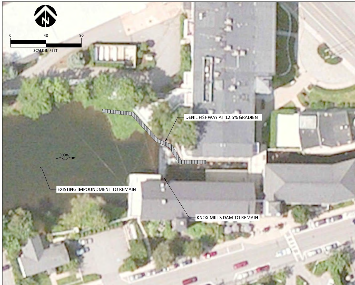
Figure 95. Schematic layout of a Denil fishway at Knox Mill Dam.
