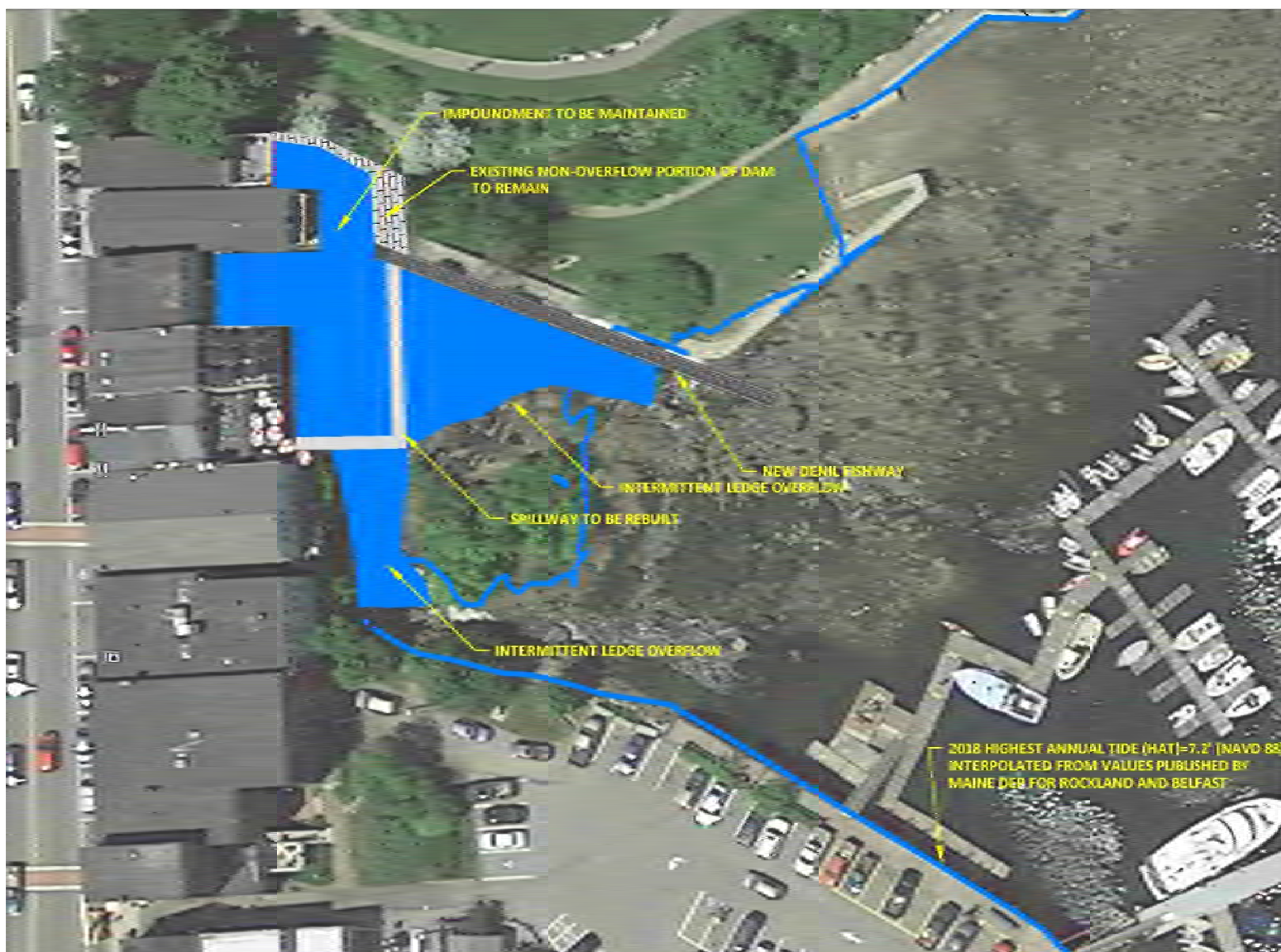
Figure 51. Schematic drawing of full spillway reconstruction with Denil fish passage along a conceptual alignment over the ledge outcrop. Imagery shown represents low tide condition (imagery source: Google Earth).
