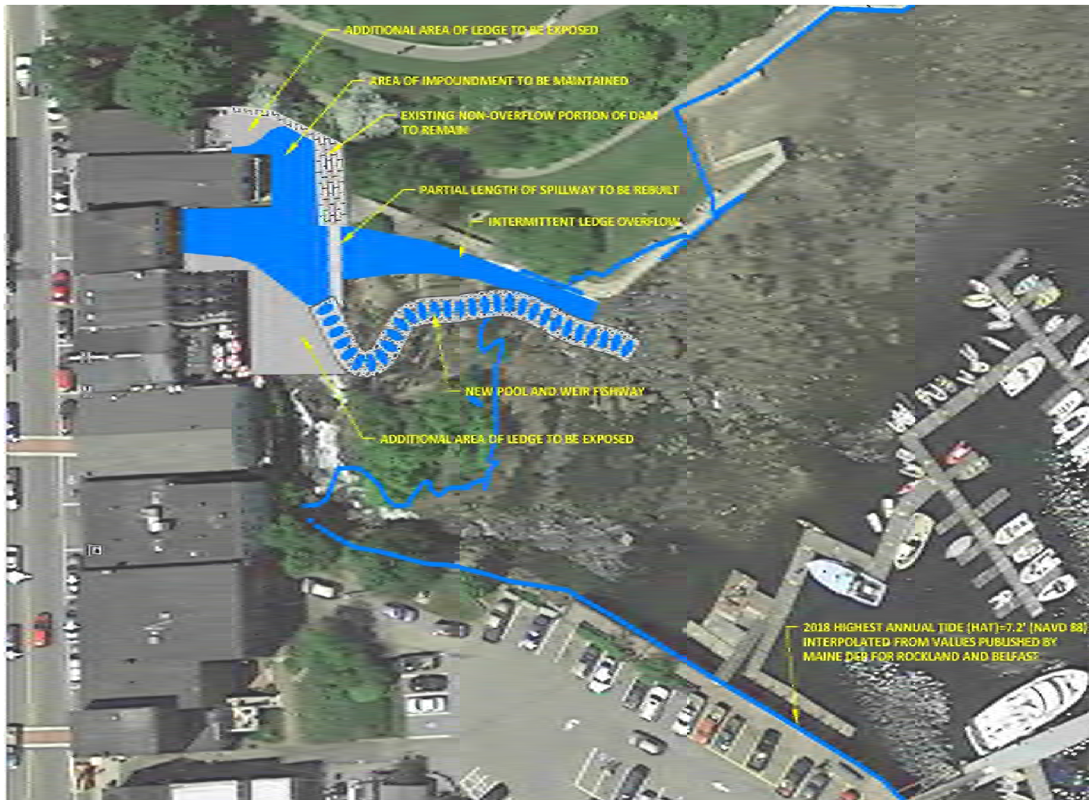
Figure 49. Schematic drawing of partial spillway reconstruction with pool and weir fishway along a conceptual alignment over the ledge outcrop. Imagery shown represents low tide condition (imagery source: Google Earth).
