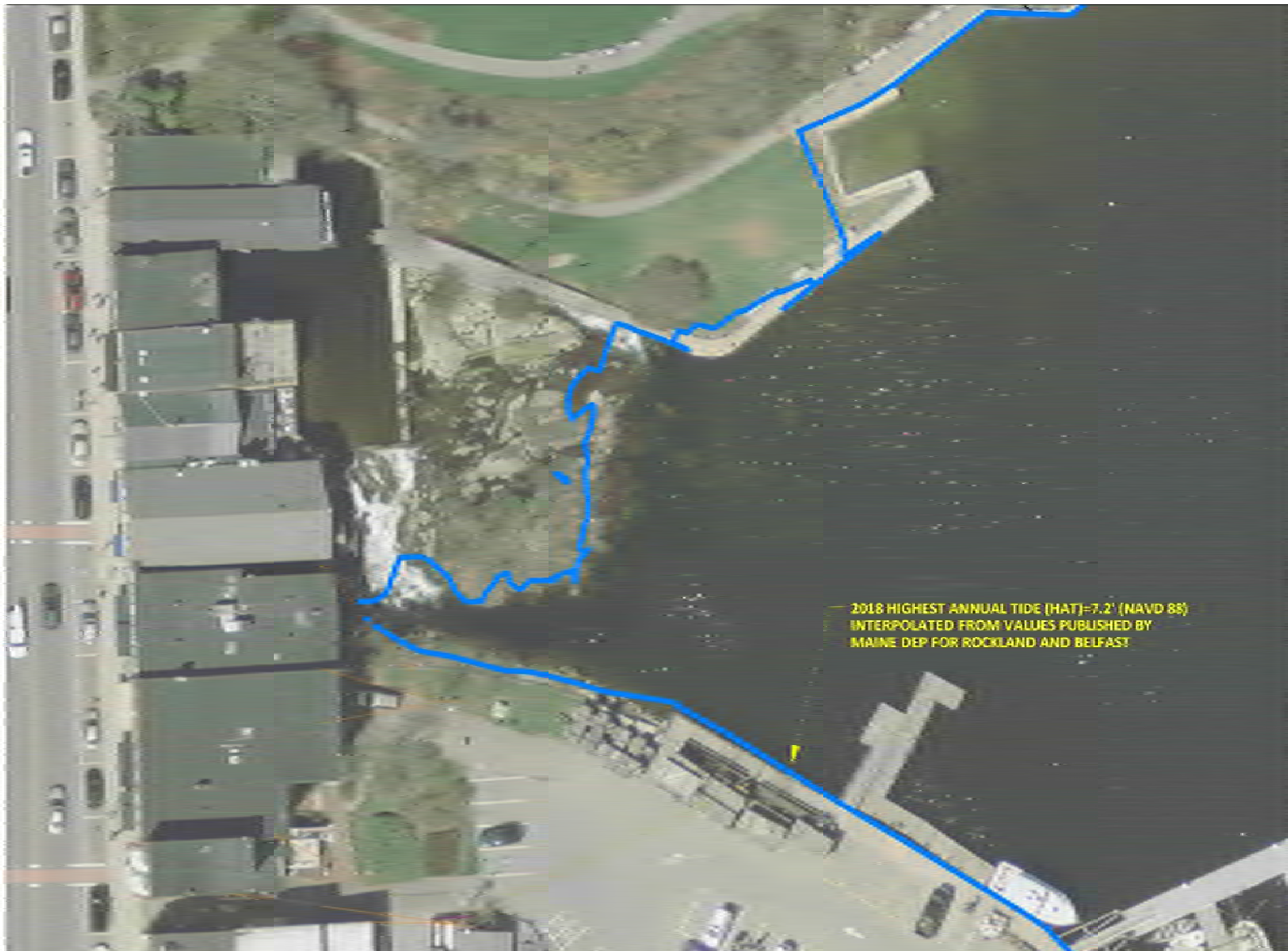
Figure 41. 2013 aerial view of Megunticook Falls and Camden Harbor showing a high tide condition (source: Maine GIS). Extreme high tides extend into the Harbor Park area over the footpath.
